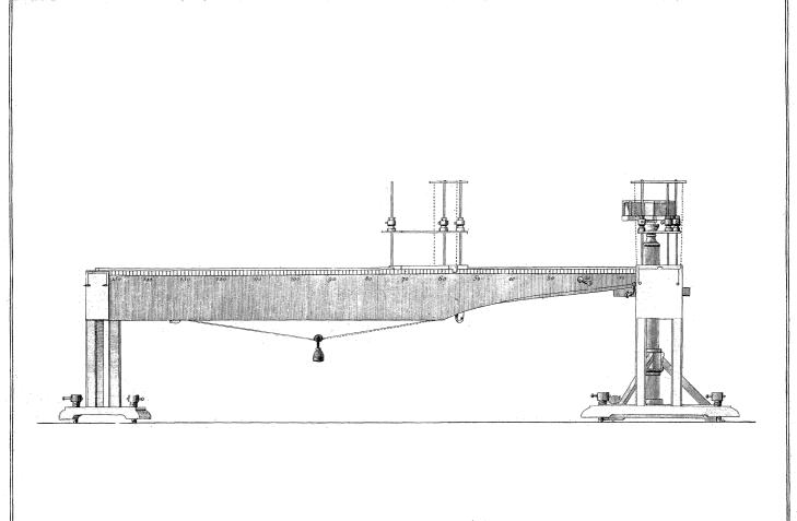
Elevation of the Photometer, with one of the Tables & Carriages.
